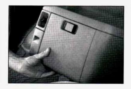
Grasp the bottom of the extension. Lift it up and then pull it out.
